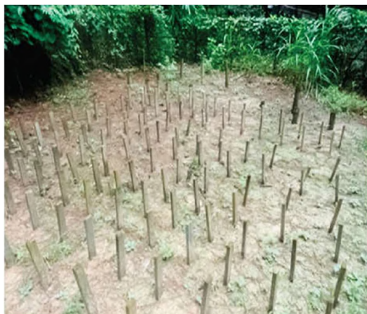
Figure 4. BRFI Stake yard
